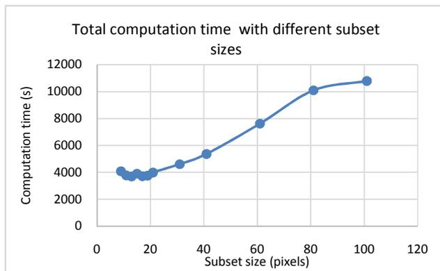
Fig. 10 Total computation time with different subset sizes
