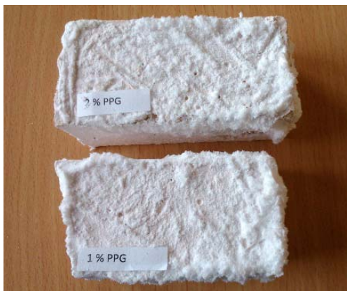
Fig. 7 Geopolymer mortar specimens containing 1 and 2% of PPG
