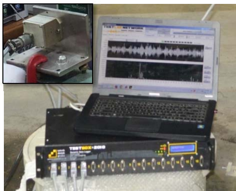
Fig. 5 Data-acquisition and Accelerometer
