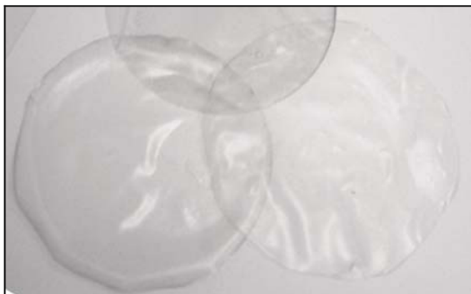
Fig. 1 A translucent starch-based film incorporated with lauric acid and chitosan
