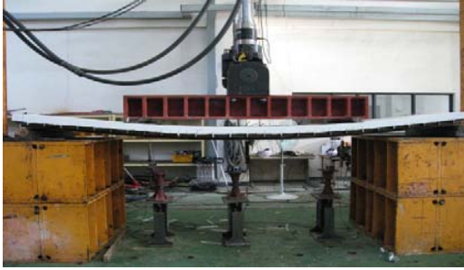
Fig. 3 Deflection under maximum loading condition
