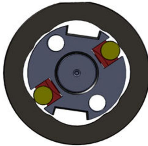
Fig. 5 Pressure course (rollers in connecting with dents of internal cam ring)
