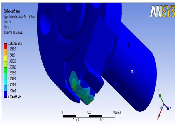
Fig. 8 Maximum stress in contact surface of roller
