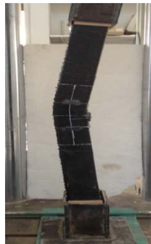
Fig. 6 Failure of CNTE specimen
