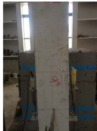
Fig. 3 Failure of control specimen
