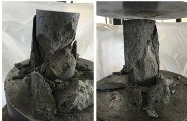
Fig. 6 Fracture aspect of 28 days compressive strength
