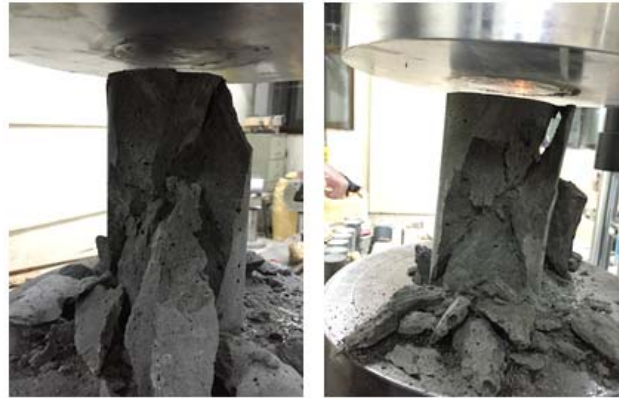
Fig. 5 Fracture aspect of 7 days compressive strength
