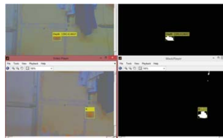
Fig. 8. Matlab Window showing Video Display Screen for pendulum oscillation where object detection is present and thus object location is detected. Here the right panes display the scene of interest in a Foreground Masked binarized format while the left panes display the scene as captured by the two Cameras
