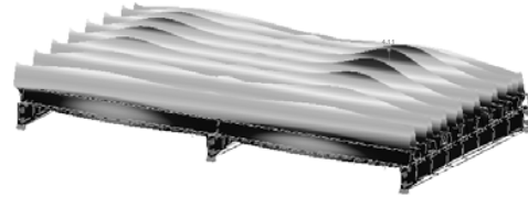
Fig. 21 Deformation (UPE 300 and Arval 420/200, L = 3 m)
