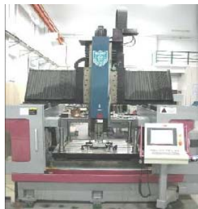
Fig. 3 NC incremental forming machine
