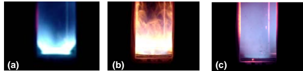
Fig. 2 Flame appearance in (a) Stable, (b) 1 st unstable and (c) 2 nd unstable operating regimes
