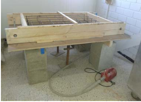
Fig. 4 Detailed reinforced floor (1.2 m×0.8 m×0.2 m) in the initial phase
