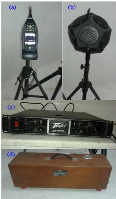
Fig. 5 Building acoustic equipment used for the measurements (a) Sound level meter Brüel and Kjær 2270 with accelerometer, (b) sound source, (c) professional signal amplifier and (d) Tapping machine
