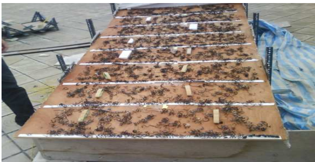
Fig. 15 Steel wire-stuffed channel (Case 5)
