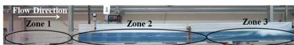
Fig. 2 Three regions of slug flow, \alpha_L=0.75 , U_{sl}=0.22 m/s and U_{sg}=5.09 m/s, Tarbiat Modares University Multiphase Flow Lab. (MFL-TMU), Test No. 6
