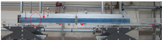
Fig. 12 Hydraulic jump at liquid holdup of 0.25 with liquid surface increase, U_{sl}=0.56\text{m/s} , U_{sg}=3.20\text{m/s} (MFL-TMU.)
