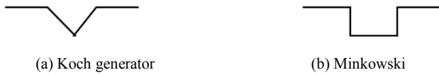
Fig. 1 Fractal curves used for the proposed antenna: (a) Koch curve along y-axis, and (b) Minkowski curve along x-axis
