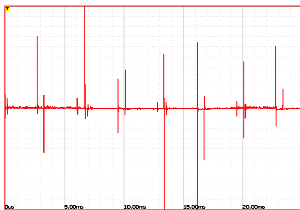
Fig. 15 Electrostatic discharges from the machine shaft
