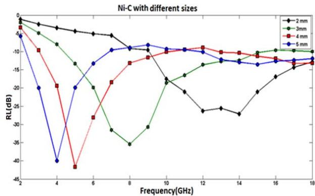
Fig. 5 The reflection loss of Ni-C with different thicknesses
