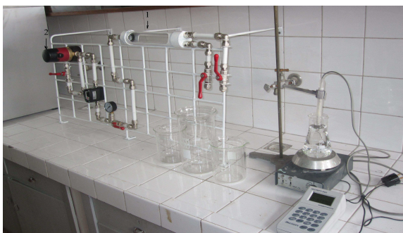
Fig. 4 Laboratory installation for the separation of emulsions using fractal systems
