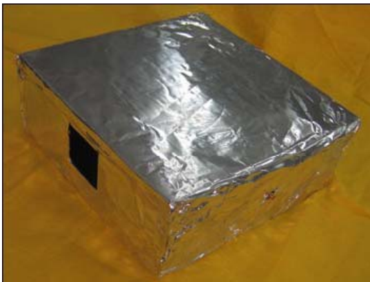
Fig. 13 The case with one aperture which is used in measurement
