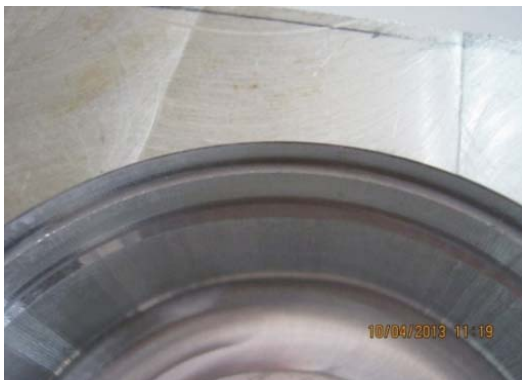
Fig. 11 Clamping Piece after Machining
