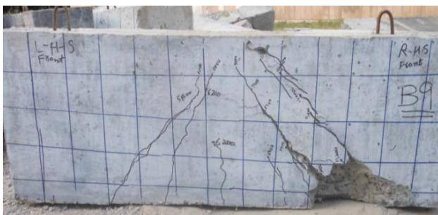
Fig. 9 457mm (18in) deep beam crack pattern
