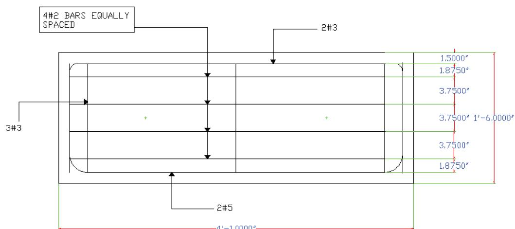
Fig. 7 Reinforcement details of 457mm (18in) deep beam
