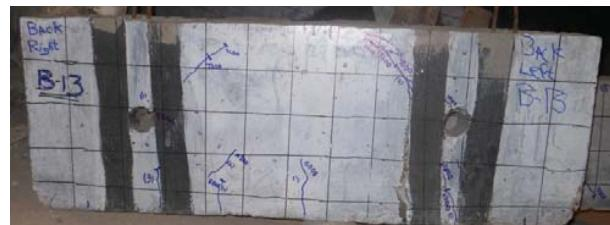
Fig. 12 Crack pattern of beams with opening at NA
