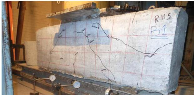
Fig. 8 381mm (15in) deep beam crack pattern
