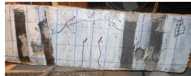
Fig. 11 Crack pattern of beams with opening below NA
