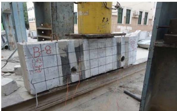
Fig. 5 Loading arrangement for beam testing
