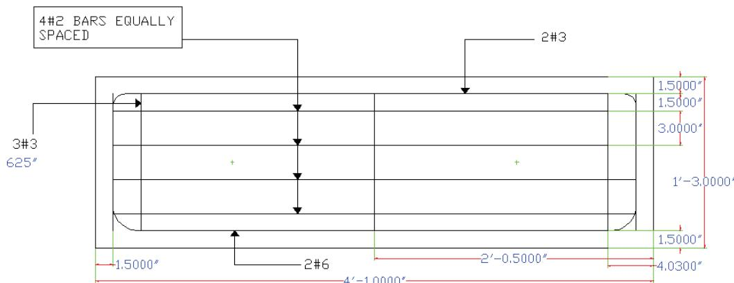
Fig. 6 Reinforcement details of 381mm (15in) deep beam
