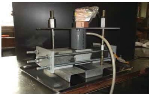
Fig. 1 Permeability test situation
