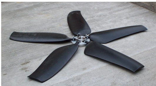
Fig. 6 A 1.618m Propeller fan wheel with 5 blades
