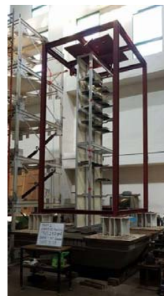
Fig. 5 STK and frame implemented on the shake table
