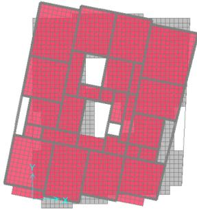
Fig. 11 (a)  $T_2=0.902$  sec (Model I) no infill wall
