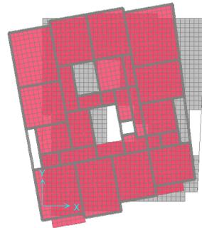
Fig. 10 (a)  $T_1=0.950$  sec (Model I) no infill wall
