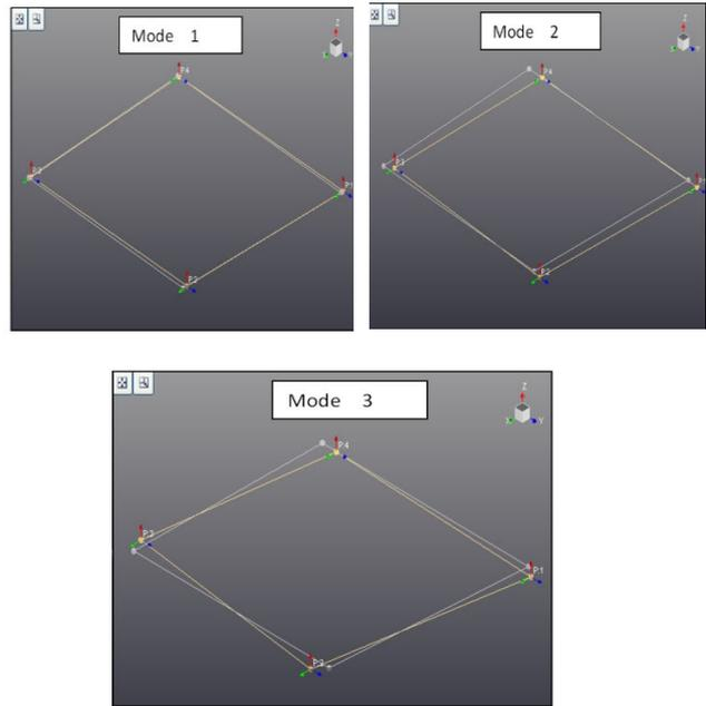
Fig. 9 Experimental mode shapes for the building
