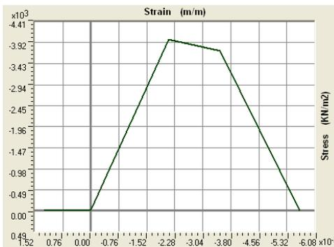
Fig. 6 (c) Stress-strain curve for clad brick
