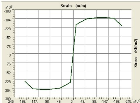
Fig. 6 (b) Stress-strain curve for steel bare
