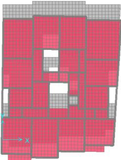
Fig. 12 (a)  $T_3=0.637$  sec (Model I) no infill wall
