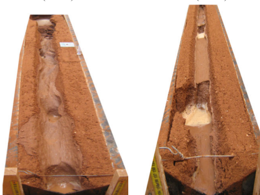
Fig. 4b Types of erosion for circular groove
