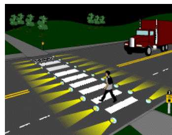
Fig. 8 In-pavement flashing warning lights [9]
