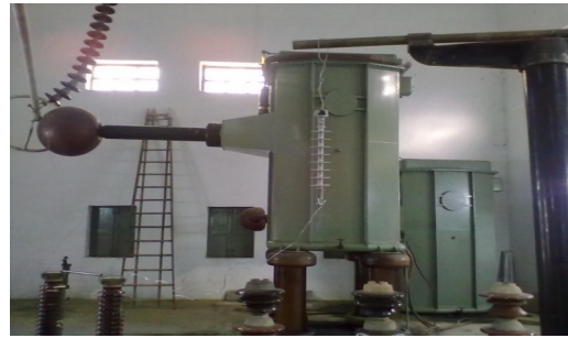
Fig. 2 Experimental arrangement of Insulator in the test
