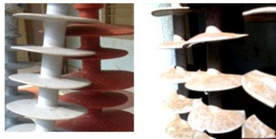
Fig. 8 33 kV Specimens under salt pollution
