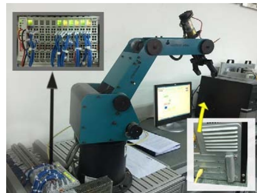
Fig. 7 Control system and robotics arm installation
