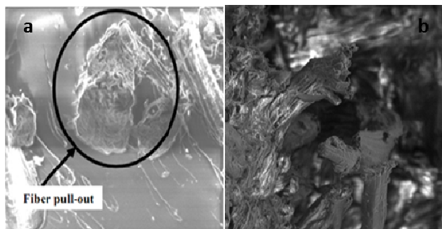
Fig. 5 Types of failure of kenaf fiber after the test; (a) 10 wt% and (b) 30 wt%
