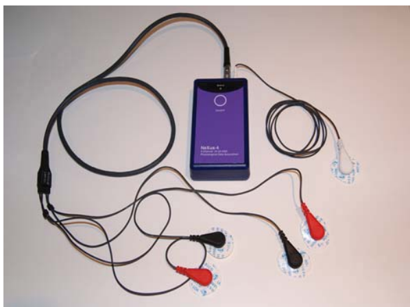
Fig. 5 Measuring electrical nerve impulses using surface-placed electrodes along jaw-line muscles [5]
