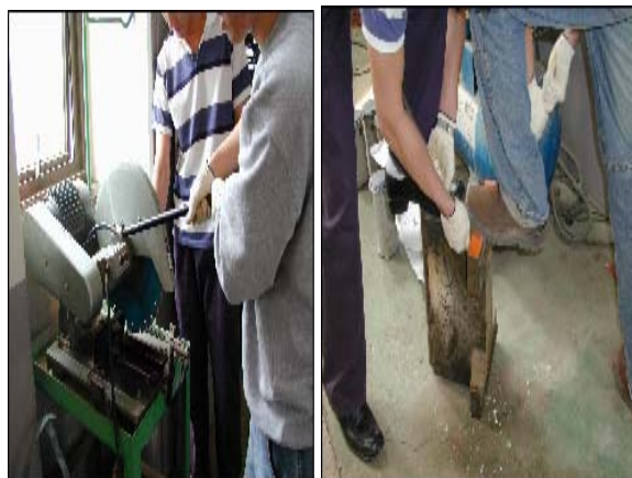
Fig. 4 Process of marking the scales to the reinforced bar staff
