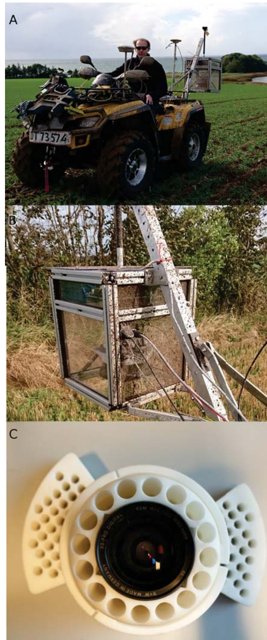
Fig. 1 (A) The ATV mounted up with RTK GNSS and the prototype camera (B) Close up of the high-speed camera after heavy rain during mapping. (C) 3D printed camera bracket
