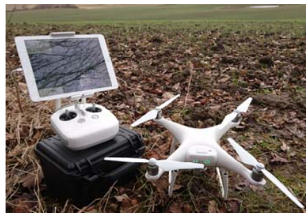
Fig. 1 Illustration of the iPad with running application and the DJI Phantom 4 Pro Drone after successful mission completion. Picture taken during test of the system on February 6, 2017
