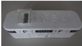
Fig. 4 RFID data logger (SL900A) on a box
