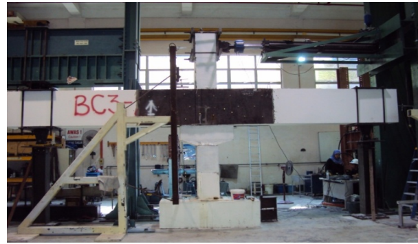
Fig. 2 The specimen BC-23ER is ready for testing
