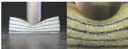
Fig 3 indentation in sandwich beam with PU core
