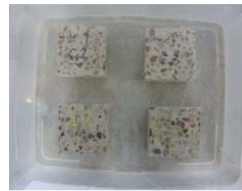
Fig. 2 Samples of the concrete immersed in the solution of H 2 SO 4 acid
