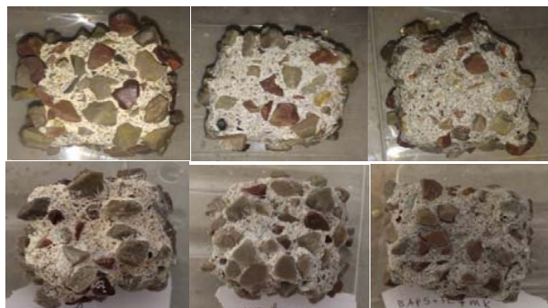
Fig. 5 The visual appearances of specimens after 8 weeks exposure to sulfuric acid solution at age of 90 days of cure
