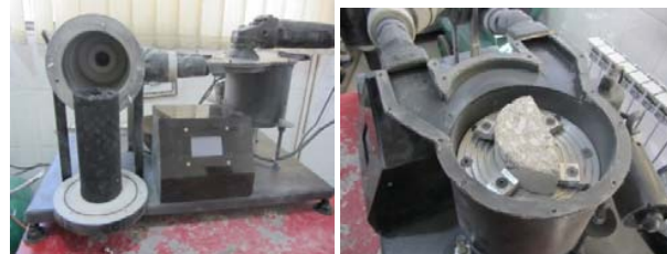
Fig. 11 The used device to obtain concrete powder samples at different depth from the exposure surface [12]
