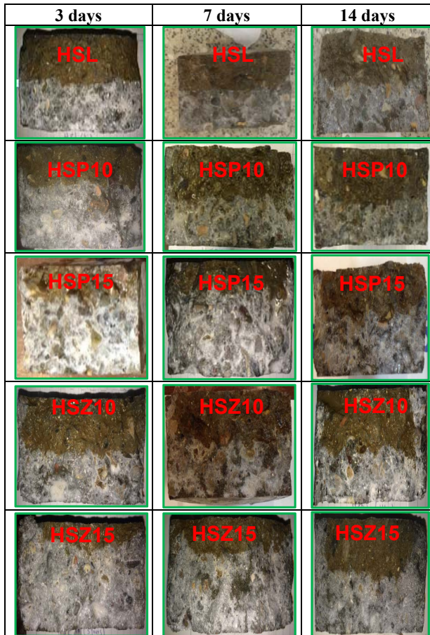
Fig. 8 Chloride penetration depth after RCMT test in the different studied HSSCCs at 3, 7, and 14 days of aging
