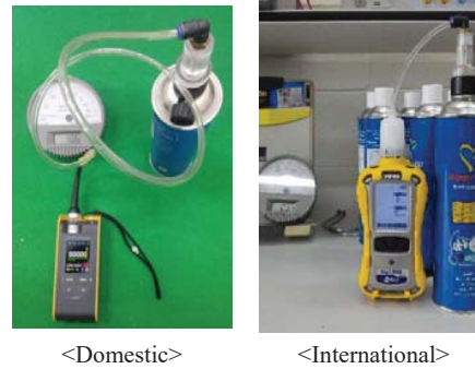
Fig. 4 Comparison Test of combustible gas detectors
