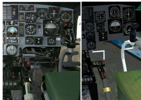
Fig. 2 A photograph of a helicopter control panel and flight controls (left) with the corresponding representation in the simulator (right)
