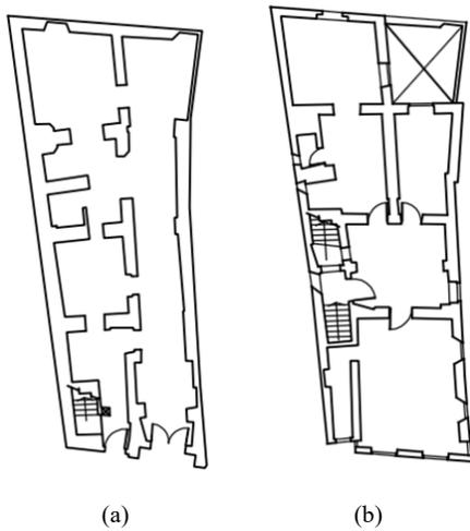
Fig. 21 (a) The existing ground floor plan and (b) existing first floor plan of Thabet House
