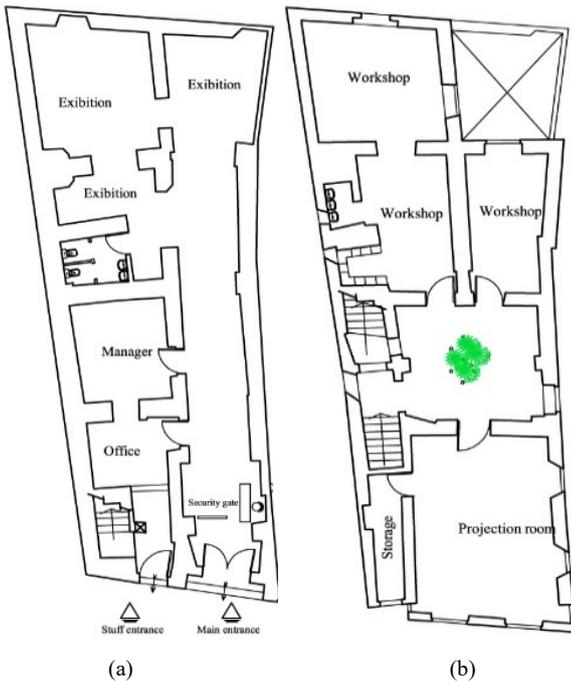
Fig. 26 (a) The proposed ground floor plan and (b) first floor plan of Thabet House
