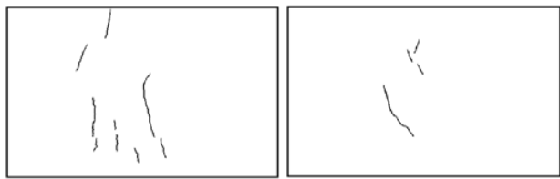
Fig. 10 Plastic shrinkage cracking 1.50% RP fiber, length 20mm
