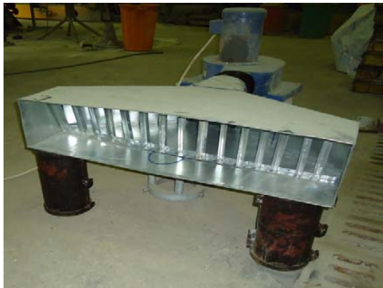
Fig. 3 Shape of directing channel for blower
