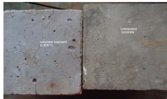
Fig. 2 Concrete exposed to 800°C
