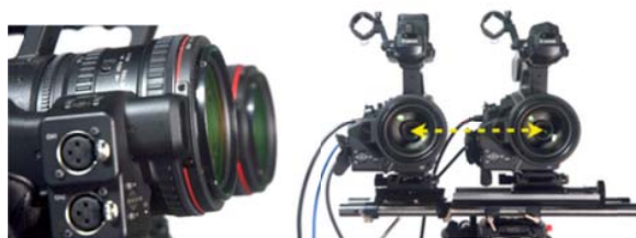
Fig. 13 Stereo camera: interaxial separation
