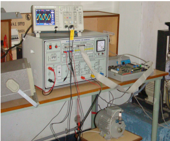
Fig. 16 Experimental setup of three-level inverter
