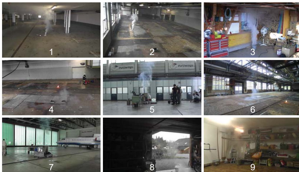
Fig. 6 Videos used for evaluation with various smoke densities. 1-3 high density, 4-6 mixed density, 7-9 low density
