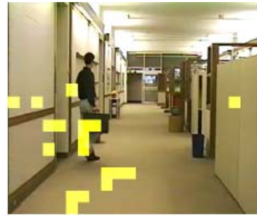
Fig. 3 Intracoded blocks indicated by yellow squares
