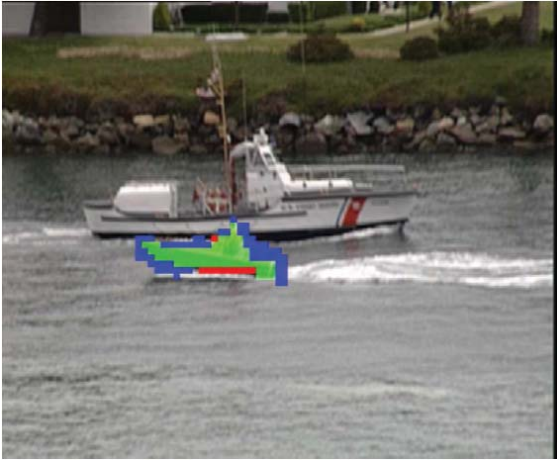
Fig. 7 Target at frame of Coastguard superimposed by scaled MV field after GMC
