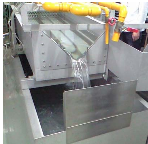
Fig. 2 Regular triangular weir of 320 mm side length
